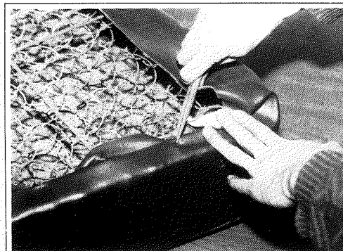
Figure 32. ...and secure. To finish off, tuck the excess material under the spring bars. Job done.
