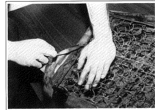
Figure 28. With the rings removed, compress the spring unit and unpeel the old fabric.
